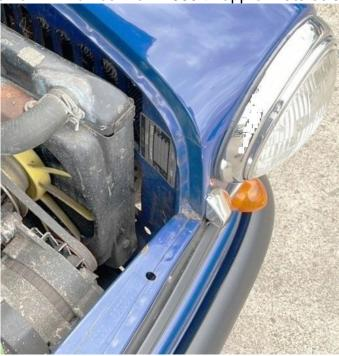
Below shows an early 90's UK car. The body number plate was on a thin embossed strip. On 1980's cars the VIN plate was on the LH inner wing
