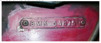
Mid 60's: The body number was generally fitted to the front panel on a welded on plate certainly on Longbridge built cars
