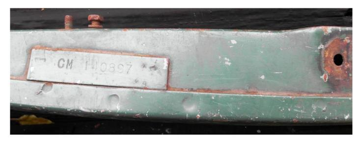
By the end of the 1960's the body number was usually (but not always)on the left hand side of the slam panel as the Chassis and Commission plates were then mounted on the right hand side of the slam panel. Mini Mokes have a different style of body number.
